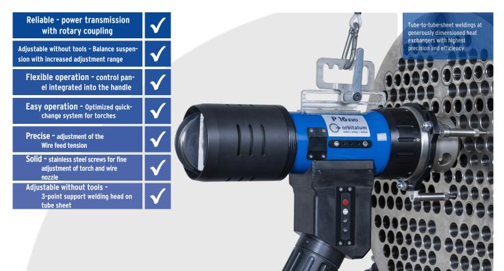
The P16 EVO TIG tube-to-tube-sheet weld head is the result of continuous further development of the proven P series. Tool-free balancing and integrated control keypad increase operating convenience. The use of high-quality components and materials raises the precise reproducibility of welds to a new level.
