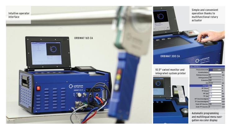
In addition to the reliable automatic programming which generates welding parameters by entering the tube diameter, wall thickness, material and welding gas all ORBIMAT CA models also include a FLOW FORCE function to reduce the pre-flow gas time when the weld heads are closed in the standard model and BUP control function with controllable, position-dependent tube internal pressure control as an optional extra.
