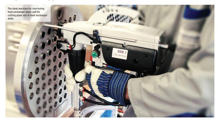
For standard-compliant, precise and reproducible weld seam preparations. The perfect addition to Orbitalum's WIG pipe-in-sheet weld heads!
